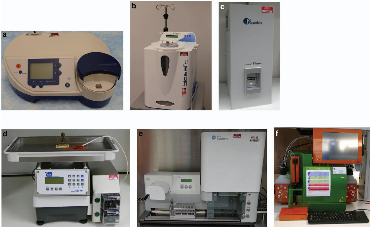
Figure 4. Equipment used during manufacture and analysis of antigen-specific T cells. (a) Amaxa Nucleofector II (AAB-1001, Lonza Group Ltd) to electrotransfer DNA plasmids into quiescent cells. (b) Biosafe Sepax II to isolate mononuclear cells from blood as well as for volume reduction procedures for large cultures. (c) Cellometer (Cellometer Vision, Nexcelom Bioscience, Lawrence, MA, USA) to automate the enumeration of viable cells. (d) WAVE Bioreactor (System 2/10 EH, GE Healthcare Bio-Sciences) to culture T cells and activating and propagating cells (AaPCs) at higher densities and volume using gas/media perfusion. (e) Vialer (Fill-It, Model 0632L10, TAP Biosystems, Sartorius Stedim Biotech Group) to automate the dispensing of cells. (f) MACSQuant Analyzer 10 (Miltenyi Biotec GmbH, Bergisch Gladbach, Germany), a benchtop flow cytometer for multiparameter cell analysis.
